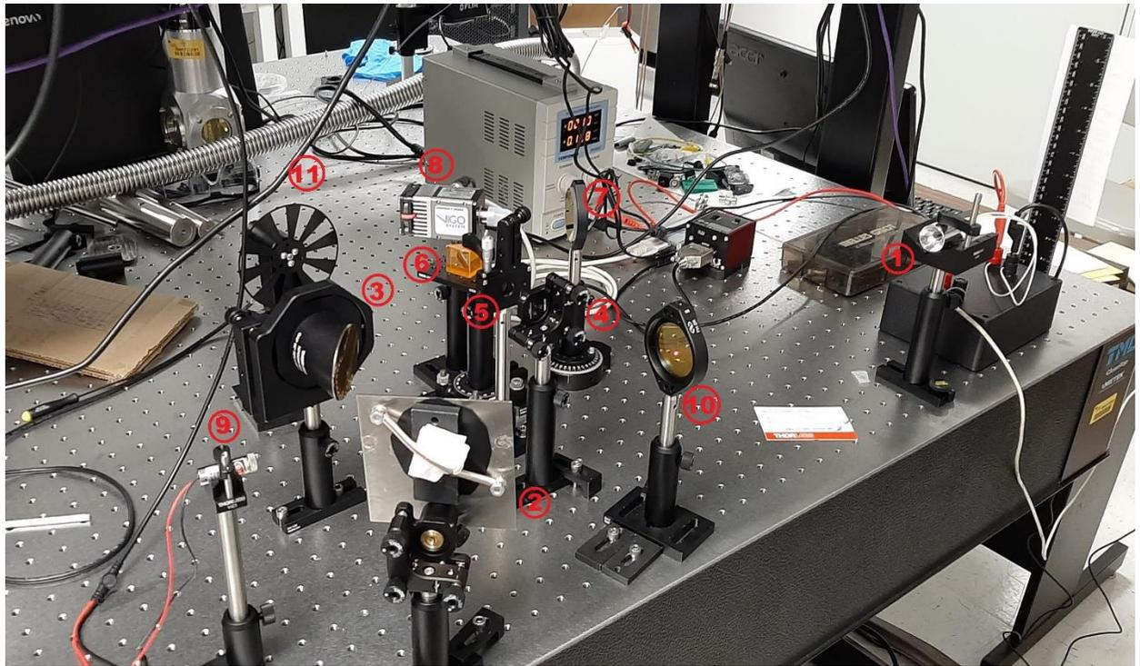
**Figure 2.** Layout of the miniaturized IR spectrometer system
